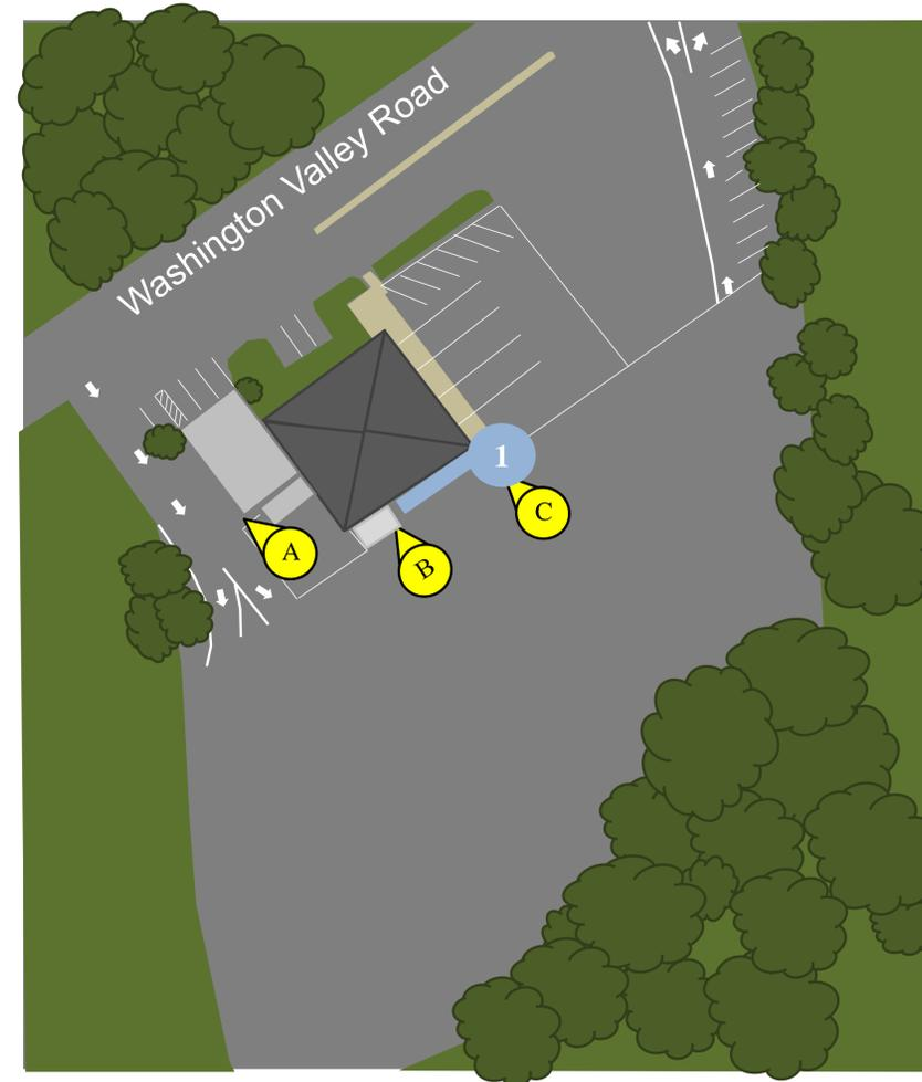
**1 RAINWATER HARVESTING SYSTEM:** Rainwater can be harvested from the roof of the building and stored in cisterns. The water can be used to wash the fire trucks.
