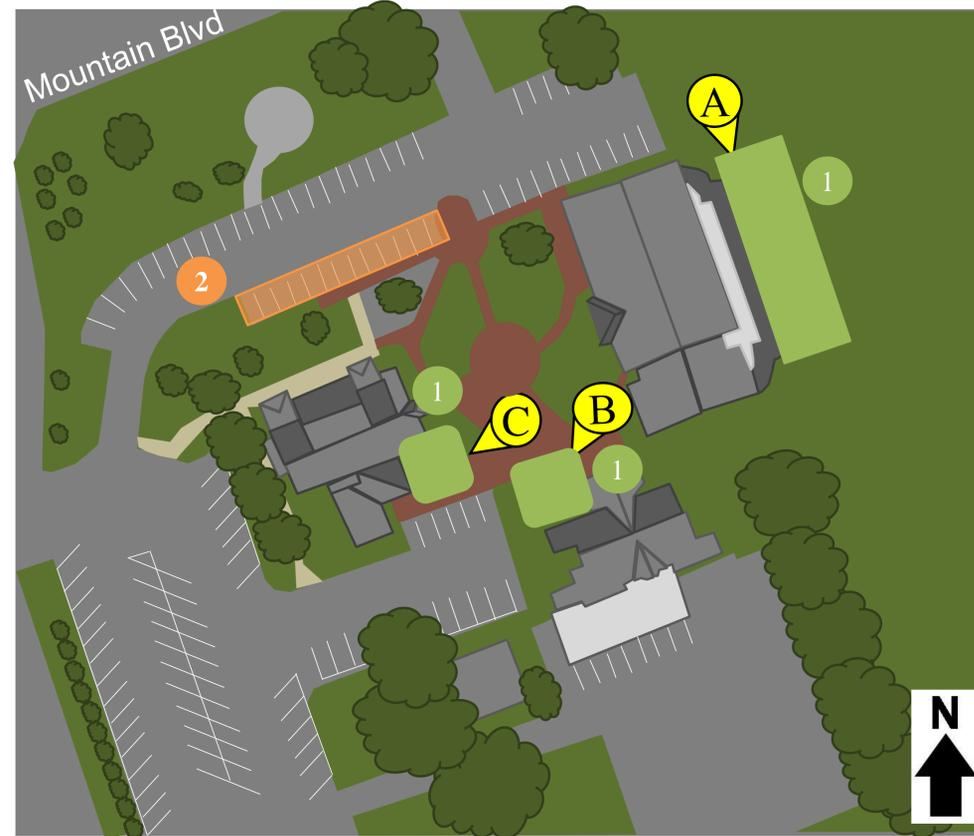
**1 BIORETENTION SYSTEM:** Bioretention systems could be installed in the large lawn on the northeast side of the library, in the grass area in the front of the court building, and near the front of the municipal building where existing downspouts can be disconnected. A bioretention system will reduce runoff and allow stormwater infiltration, decreasing the amount of contaminants that reach catch basins.
